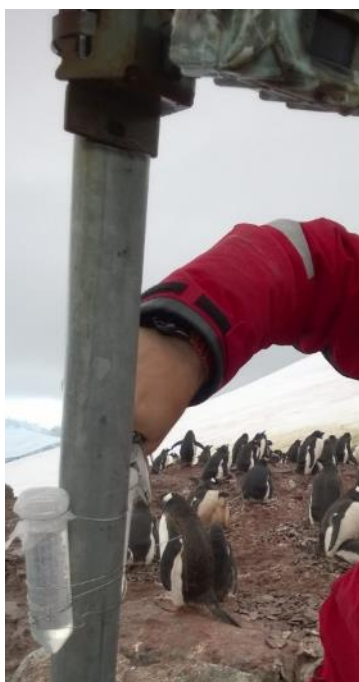
Figure 7: A camera pole with a trial pollen trap on. These traps consist of sample tubes tied to the camera pole and filled with glycerol. These tubes are covered with a filter and left for one year.
